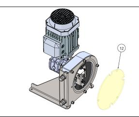
**Fig. 3.8.3** Remove the front cover [12].
