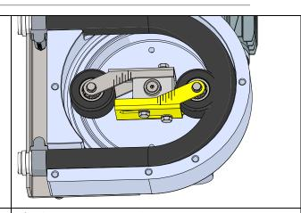
**Fig. 3.8.5a PTL9 – PTL25**On the side where the roller IS pressing the hose, loosen the roller bracket mounting screws [941] and retract the bracket so that there is no pressure on the
