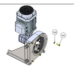
**Fig. 3.6.3** Unscrew the front connection bracket screws [141], and remove them with their washers [142].
