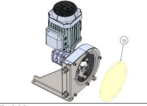
Fig. 3.6.2 Remove the front cover [12].
