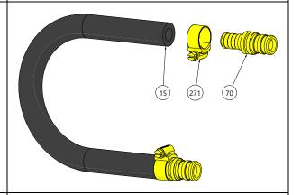
**Fig. 3.6.6** Remove the clamp bands [271] and the inserts [70] form the hose.
