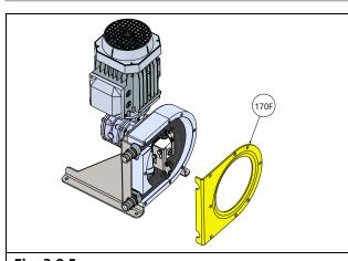
**Fig. 3.8.5** Remove the front connection bracket [170F].
