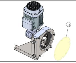
Fig. 3.8.16 Assemble the front connection bracket and the front cover [12].
