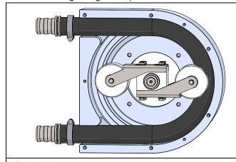
**Fig. 3.8.1**Run the pump and position the rotor so that only one roller is pressing against the hose.
