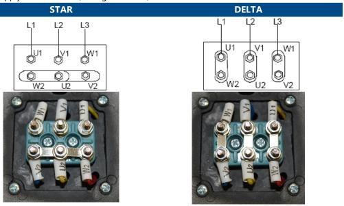
Follow the connection standard used in the plant. In no case connect the electrical motor directly to supply network but use a suitable electric switchboard equipped with a knife switch and suitable safety devices (e.g. motor breaker switches) in the power circuit. Safety devices against overloads must also protect the motors. Make sure that the motor has suitable grounding and that it has been connected properly.
