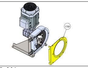
**Fig. 3.6.4** Remove the front connection bracket [170F].
