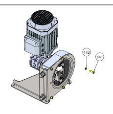
**Fig. 3.8.4** Unscrew the front connection bracket screws [141] and remove them with their washers [142].
