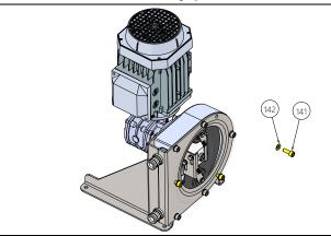
**Fig. 3.6.1** Unscrew the front cover mounting screws [141], and remove them with their washers [142].
