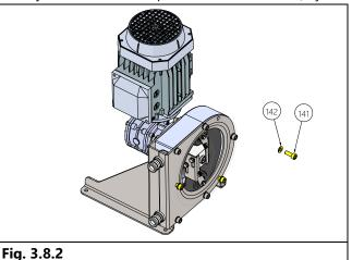
Disconnect power supply from the motor. Unscrew the front cover mounting screws [141] and remove them with their washers [142].
