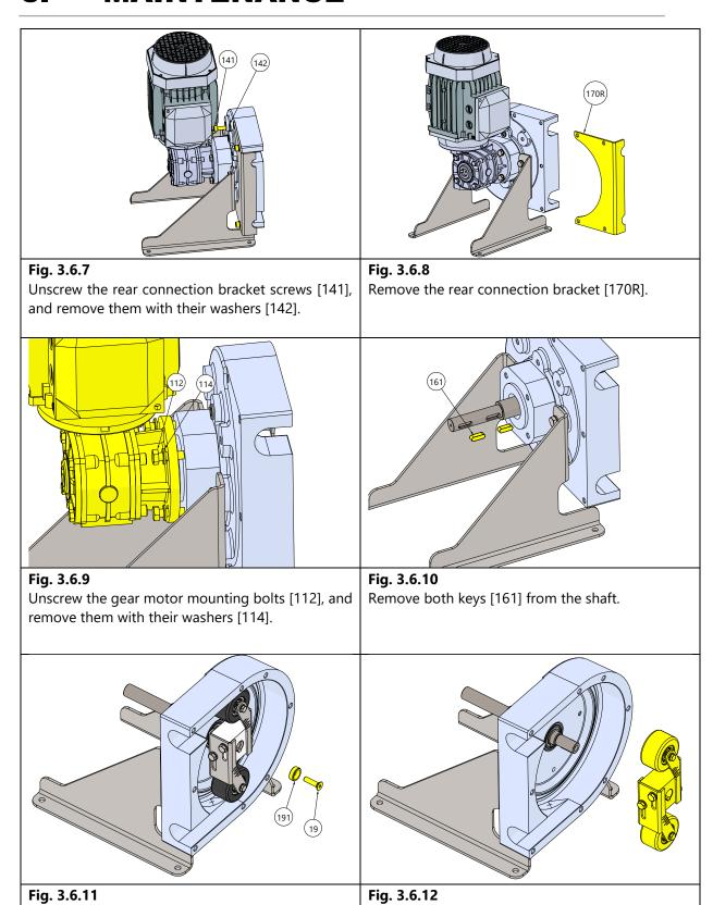
Remove the complete rotor/roller assembly.
