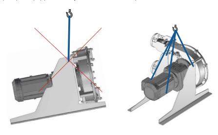
Never lift the pump under pressure.
