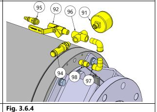
Remove the pneumatic fittings from the dampener.
