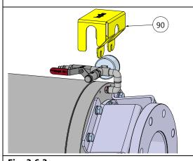
**Fig. 3.6.3**Remove the pneumatic fittings cover [90] from the dampener.
