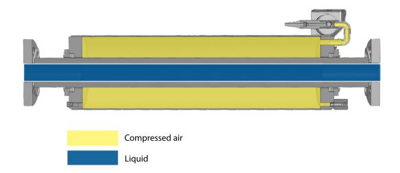
The air pressure supplied to the dampener must be equal to 85% of the pump discharge pressure. The medium flowing through the dampener affects the hose, which by means of the compressed air on the air side compensates the fluctuations of pressure in the discharge line. The air concentrated in the dampeners block works as a spring for the medium flowing through the dampener.
